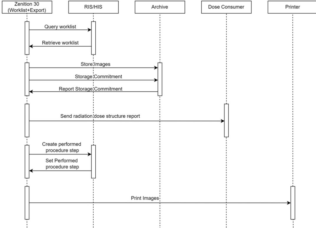
**Figure 3: Typical Acquisition Archive Storage Sequencing Constraint.**
