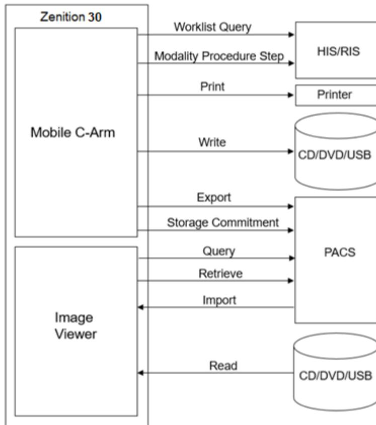
Figure 1: System Overview of Mobile C-Arm with integrated Image Viewer
